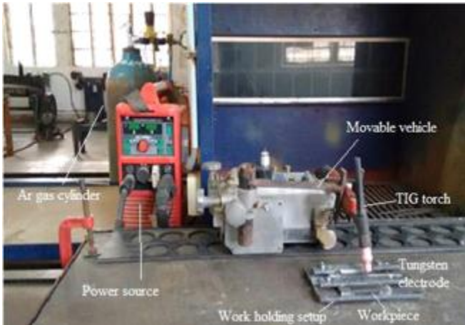
Fig. Experimental setup of TIG welding
