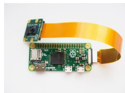
Fig -3.6 Camera module attached to Raspberry Pi
