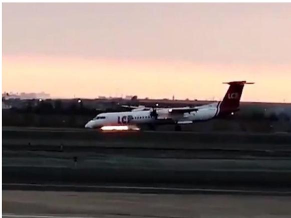
Fig-4: Landing Gear Failure
