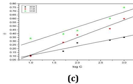
Fig. 3 (a) Langmuir, (b) Frumkin, (c) Temkin isotherm for the adsorption of SAL inhibitor on MACS in 1.0N HCl.
