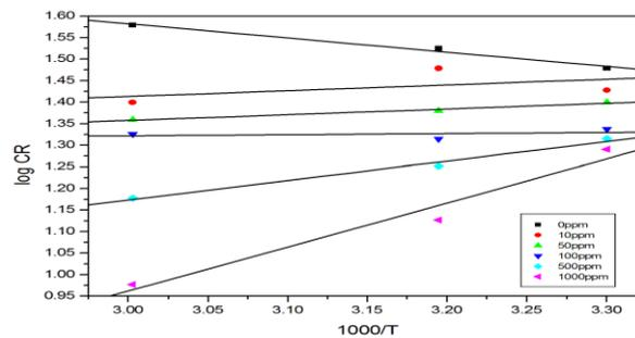
**Fig-1. Arrhenius plot for MACS corrosion 1.0N HCl in the absence and presence of different concentration of SAL.**
