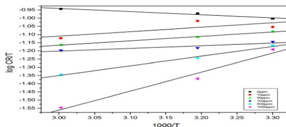
**Figure-2 Transition state plot for MACS corrosion in 1.0N HCl in the absence & presence of different concentration of SAL.**
