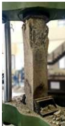
Fig-3: Compression test on RCC columns after fire
