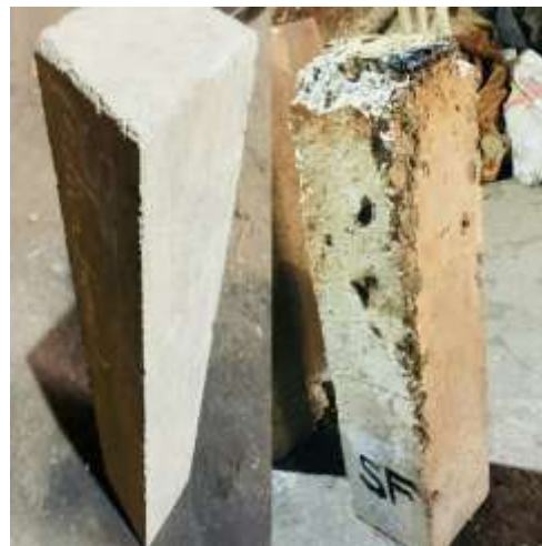
Fig-4: Spalling of column before and after
