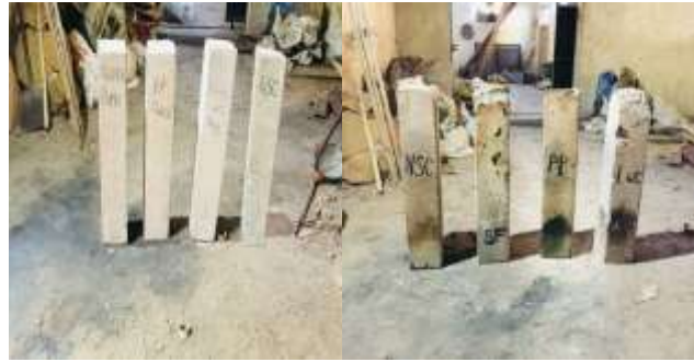
Fig -4: HSC and NSC column after fire
