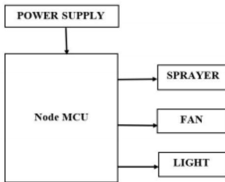
Fig -2: Block diagram of control part
