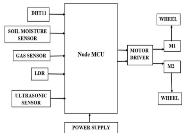
Fig -1: Block diagram of vehicle part
