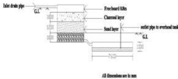
Fig-2: Plan of the Filtration Tank
