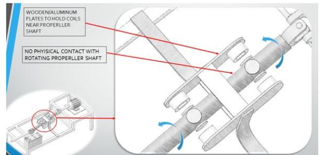
**Fig-3:** Close view of magnet arrangement
