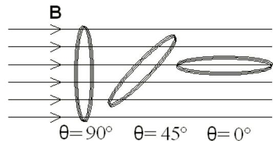
Fig-5: Field Lines through Coils
