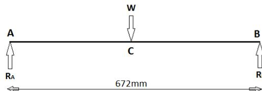
Fig- 4: Vertical loading diagram of shaft
