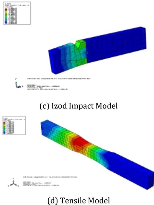
**Fig-4:** Compression, Flexural, Izod- Impact and Tensile Failure Models
