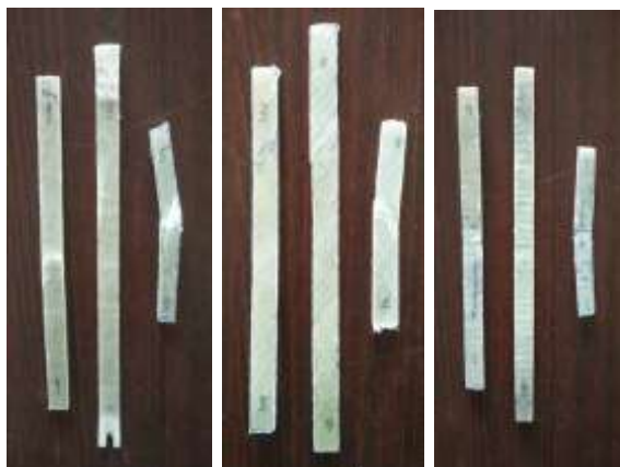
Fig -2: Fractured Test Specimens
