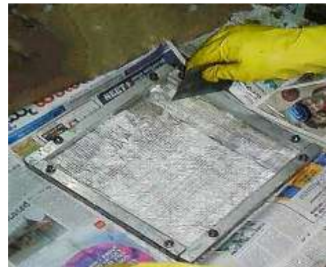
Fig -1: Manufacture of glass fiber laminates using Hand layup method
