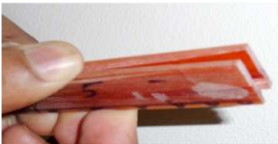
Fig-12: (b) Delamination Due to Release Film
