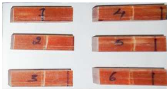
Fig- 15 ILSS Specimens After Test
