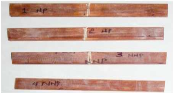
Fig- 12: (a) Flexural Specimens After Test
