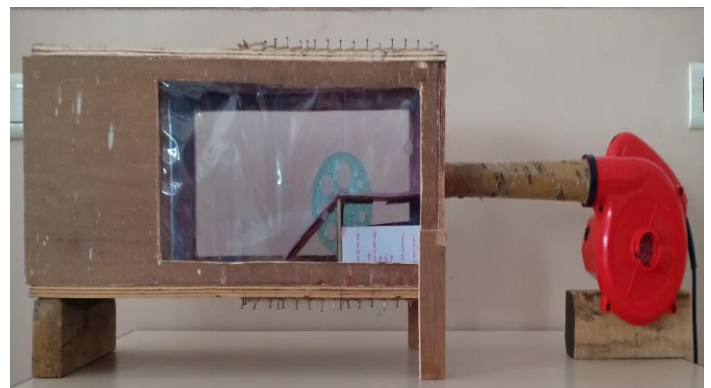
Fig. 4.1 Experimental Set-Up with angled flat surface
