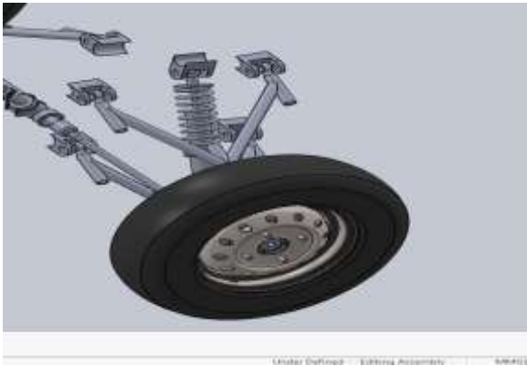
Fig - 6 : Front a-arms with suspension
