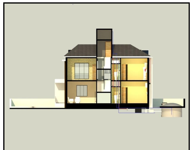
Fig -11: Placement of rainwater harvesting tank
