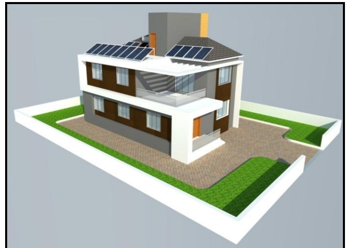
Fig -9: Arrangement of solar panels
