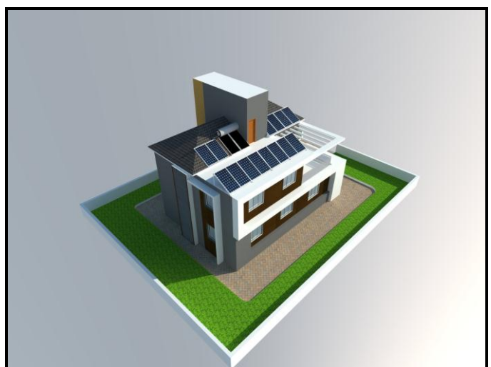
Fig -10: Arrangement of solar water heater
