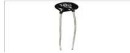
Fig (3.4) Temperature sensor
