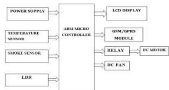
Fig(3.1). System block diagram
