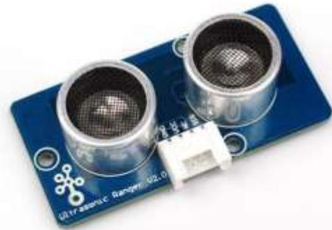
Fig -4: Ultrasonic Sensor
