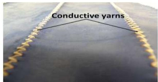
Fig -5: Conductive Yarn
