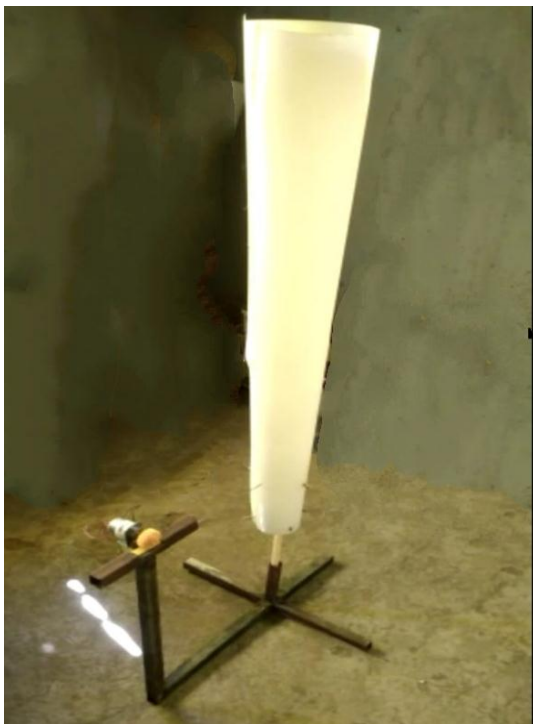
Fig-4: Actual Setup of vortex bladless windmill with mechanical arrangement
