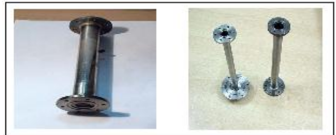
Fig.1: Typical pictures of Regenerator and Pulse tube
