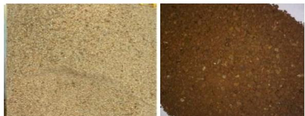
Fig 1: River sand and Excavated soil
