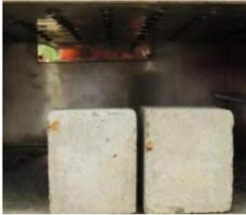
Fig 3: Thermal test on concrete
