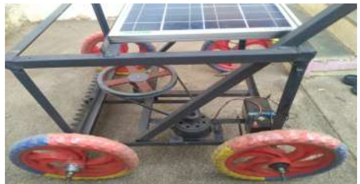
Fig-1: Side view of Solar Economical grass cutter
