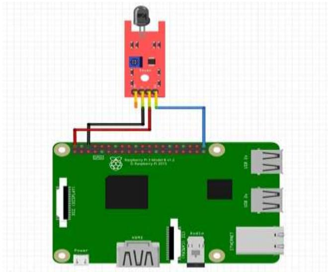
**Fig -4.2:** Connecting Flame Sensor with Raspberry Pi
