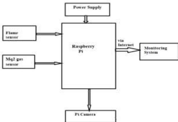
**Fig -3.1:** Block Diagram of the Proposed System
