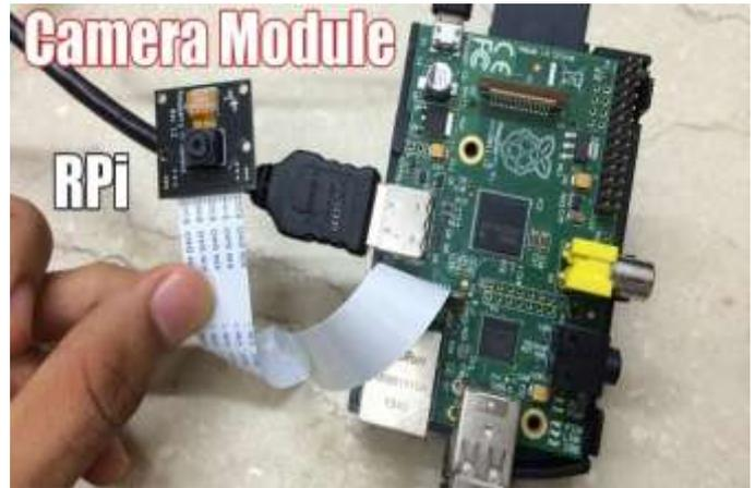
**Fig -4.3:** Connecting Pi Camera to Raspberry pi
