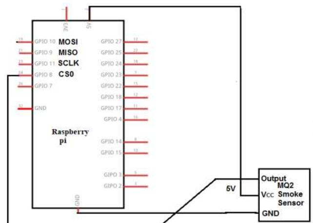
**Fig - 4.1:** Connecting MQ2 Sensor to Raspberry Pi
