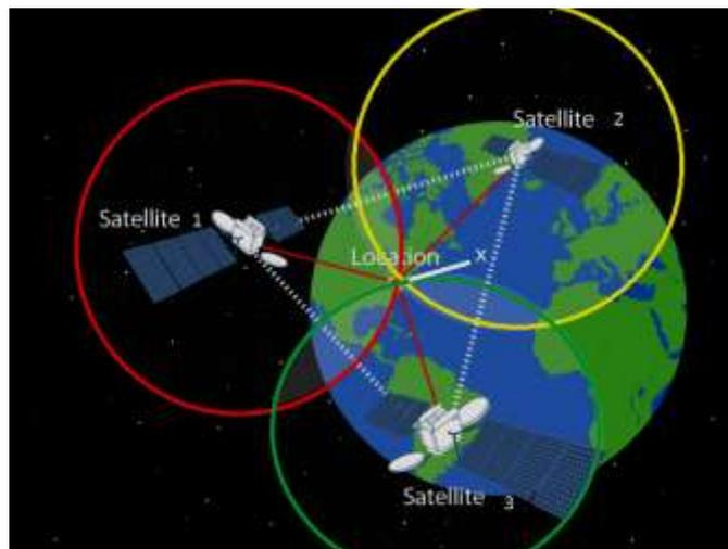
In geometry, **trilateration** is defined as the process of determining absolute or relative locations of points by measurement of distances, using the geometry of circles, spheres or triangles.
