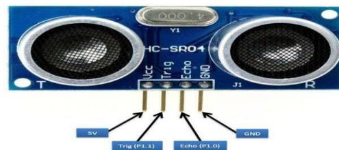
Fig. 5: Ultrasonic sensor
