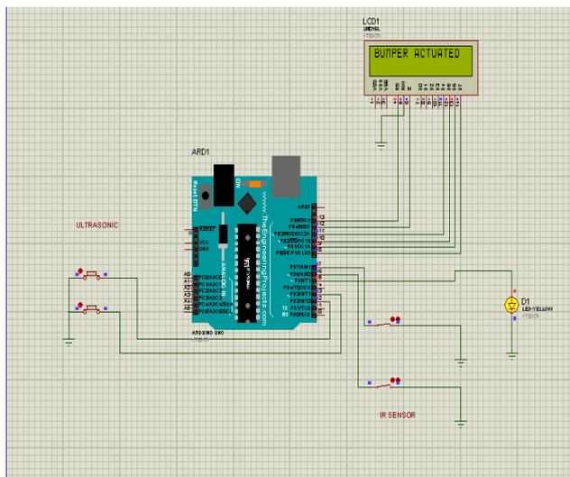
Fig. 2: Arduino Simulation (Bumper Actuated condition)
