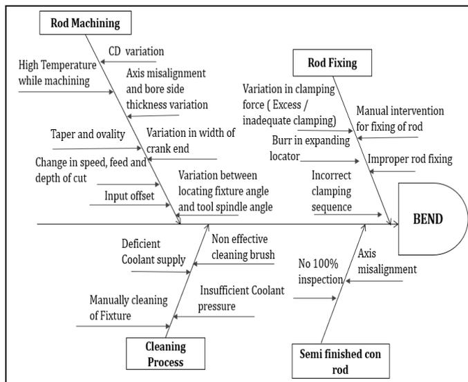
Fig -2: Cause and effect diagram
