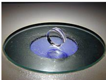
Fig-2: PDMS cylinder on the glass of a stereomicroscope light
