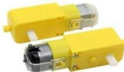
3 Volts single shaft geared motor is used as hub motor for prototype made. This motor as 150 rpm at no load condition. This motors operate at 3v-9v.
