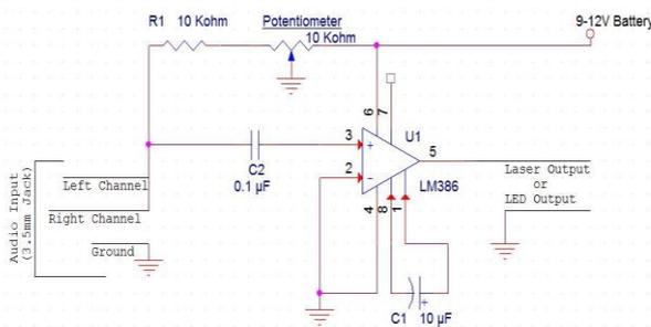
Fig -10: Transmitter Circuit
