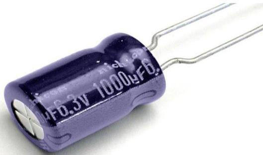
Fig -4: Electrolytic capacitor
