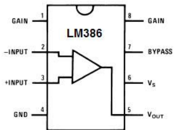
Fig -3: IC-LM386 Pin Configuration
