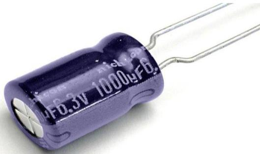
Fig -4: Electrolytic capacitor
