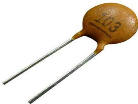
Fig -5: Ceramic capacitor
