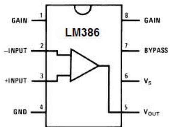
Fig -3: IC-LM386 Pin Configuration
