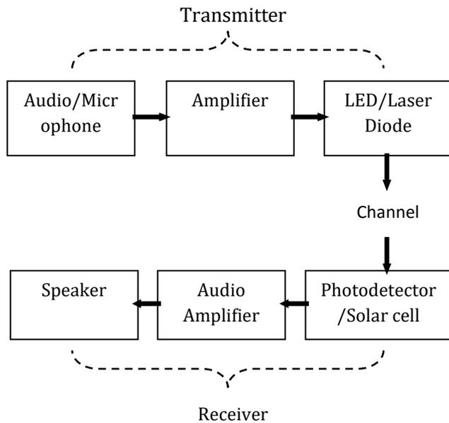
The block diagram of FSO is shown above. It can be divided into two parts – transmitter and receiver.
