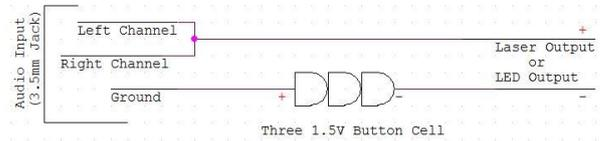
Fig -12: Transmitter Circuit
