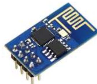
It employs a 32-bit RISC CPU based on the Tensilica Xtensa L106 running at 80 MHz (or over clocked to 160 MHz). It has a 64 KB boot ROM, 64 KB instruction RAM and 96 KB data RAM. External flash memory can be accessed through SPI.
