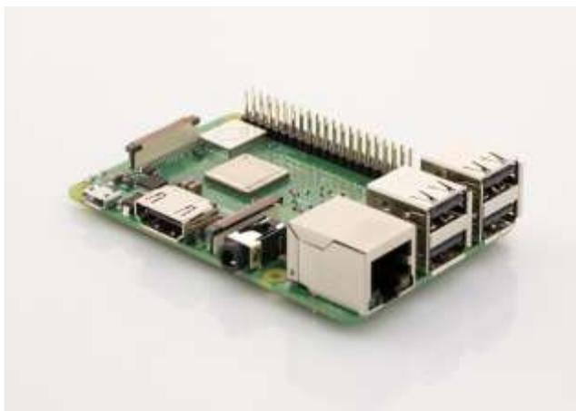
Fig -1.Raspberry Pi 3B+ model
