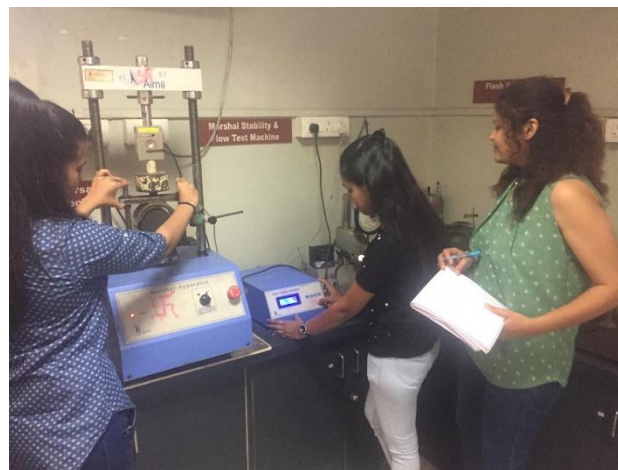
Figure 2: Testing of mould in marshall test equipment
