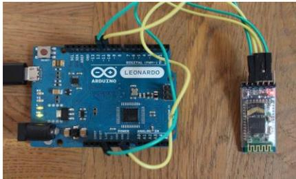
Fig -3: Bluetooth HC-05 and Arduino
