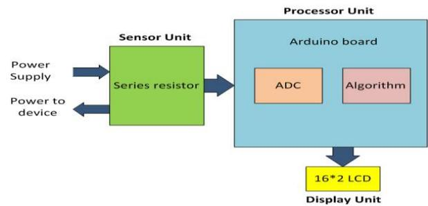
Fig -4: Block diagram
