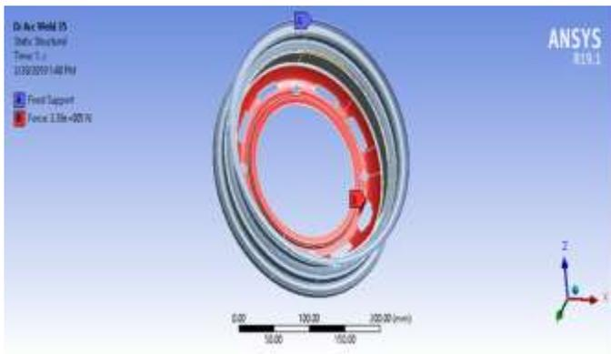
Fig -8: Weld Strength Test Boundary Conditions
