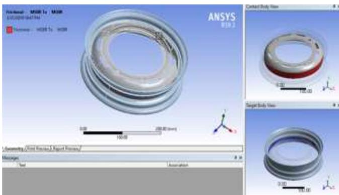
Fig -5: Frictional Contact between Circumference of Disc and Rim
