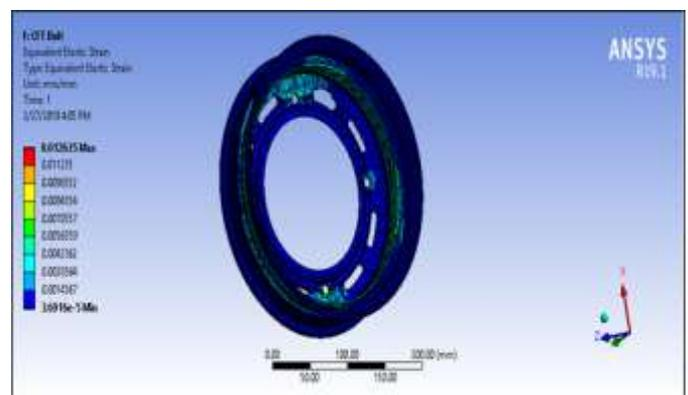
Fig -13: Strain Result of CFT (Bolt as Fixed Support)
