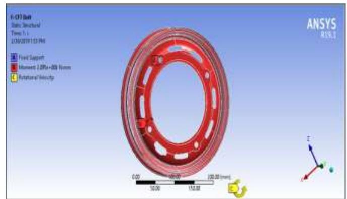
Fig -12: Boundary Conditions of CFT (Bolt as Fixed Support)
