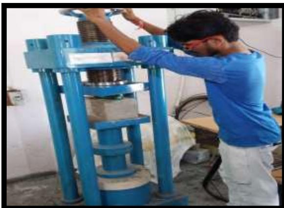
**Fig 3:** Test applied on a waste PET bottles filled with soil and sealed tightly
