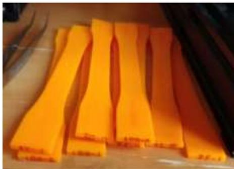
**Fig-3:** Finishing of specimen
