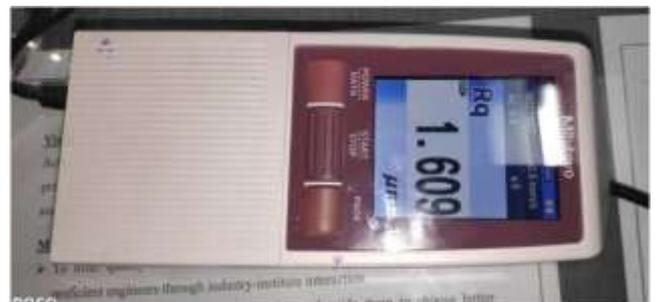
**Fig-6:** Surface Roughness Test
