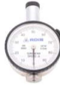
**Fig-5:** Shore-A Durometer.
