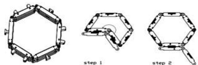
**Fig -5:** Design of a planar hexagonal module and module motion using electromagnetic coupling [22]
