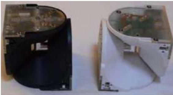
**Fig -15:** UBot active module in black and passive module in white [44]
