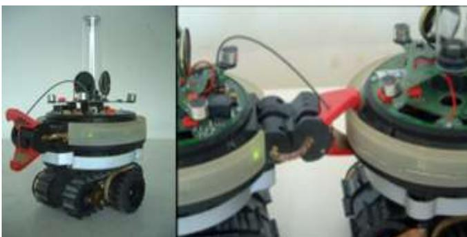
**Fig -16:** The S-Bot and S-Bot connection mechanism [47]
