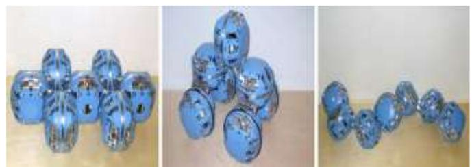
**Fig -9:** ATRON robot different configurations capabilities [20]
