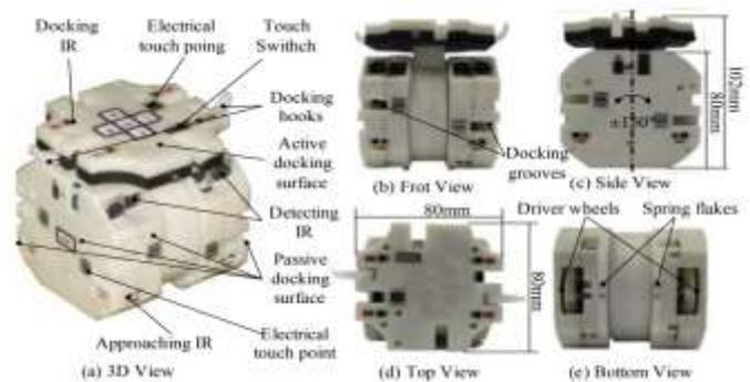
**Fig -17:** The Sambot schematic diagram [50]
