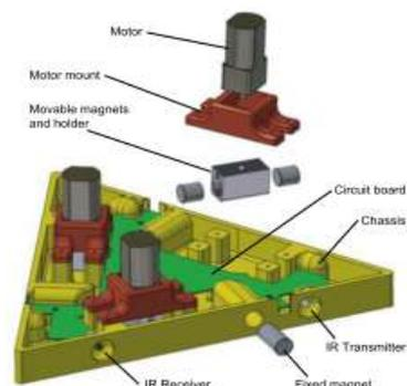
Fig -20: The component of Programmable Parts [61]
