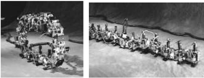
**Fig -2:** PolyBot versatile locomotion (left) rolling track; (right) snake-like locomotion [12]
