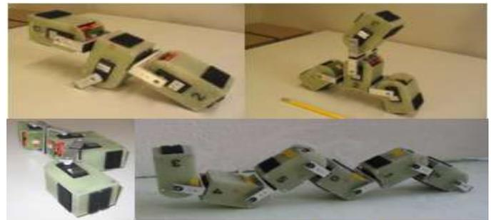
**Fig -4:** Different configuration of YaMoR robot [18]
