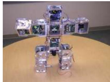
Fig -14: A network of SuperBot modules [41]
