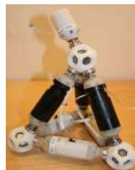
**Fig -18:** Representation of ODIN modular robot [52]
