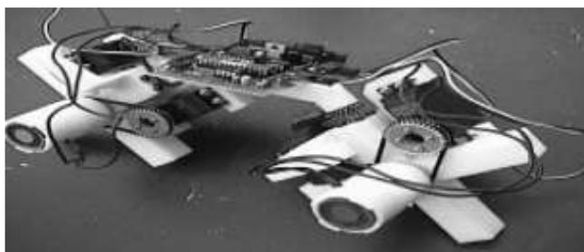
**Fig -7:** The molecule robot consists of two atoms and a right angle rigid bond binding them [26]
