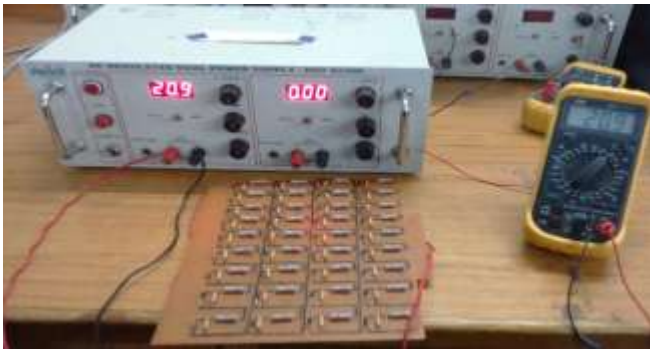
Fig.11 Measurement of Voc practically
