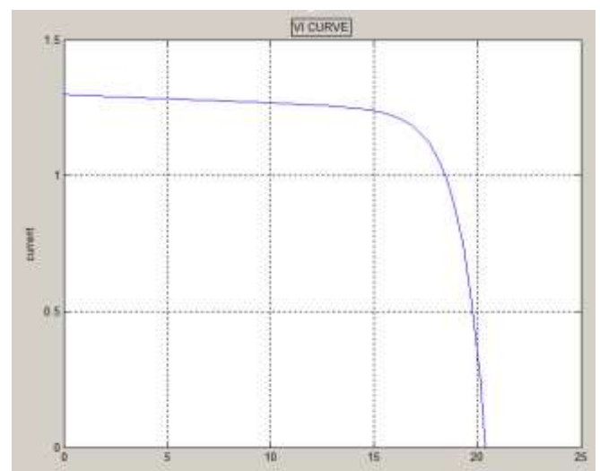
Fig.18 IV curve obtained from mathematical model
