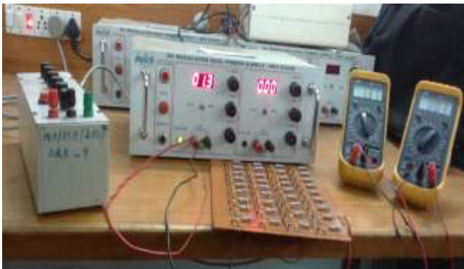
Fig.12 Measurement of Isc practically
