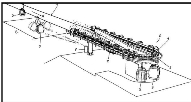
Fig -2: Turning point station
