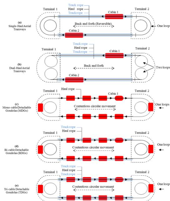
Fig -3: Detailed illustrations of RTS technologies IRJET
