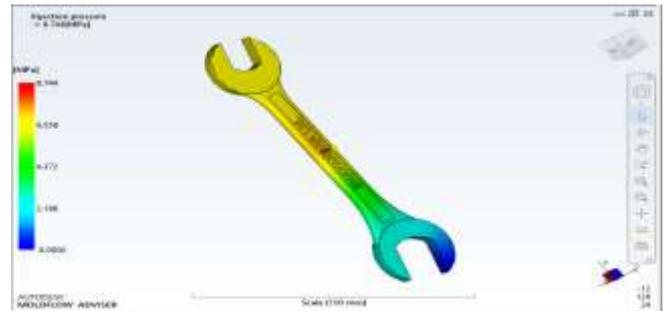
**Fig 4.7 Injection pressure at gate location 1**
