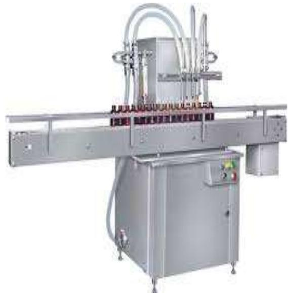
Fig4. Automatic liquid filling ladder [15]
