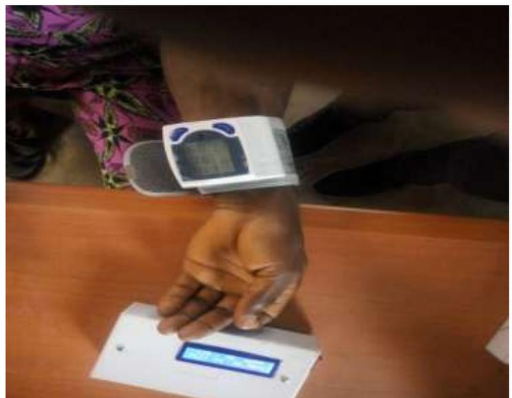
Fig 7 : HBR, BP and Temp Measurement with the Constructed Wireless Monitoring Device.
