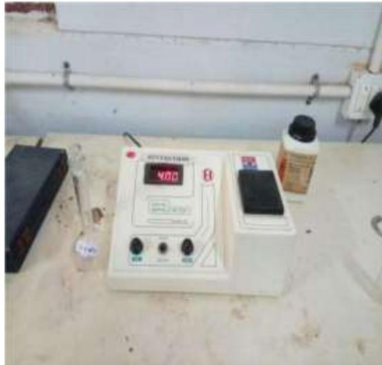
Turbidity is the cloudiness or haziness of a fluid caused by large numbers of individual particles that are generally invisible to the naked eye, similar to smoke in air. The measurement of turbidity is a key test of water quality.
