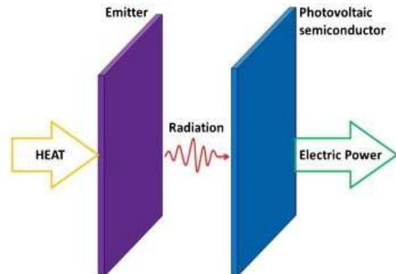
Figure 1: Basic schematic diagram of a TPV system [2]
