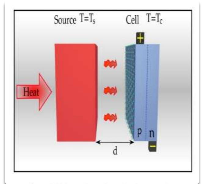
Figure 4: Near Field Thermophotovoltaics system[24]
