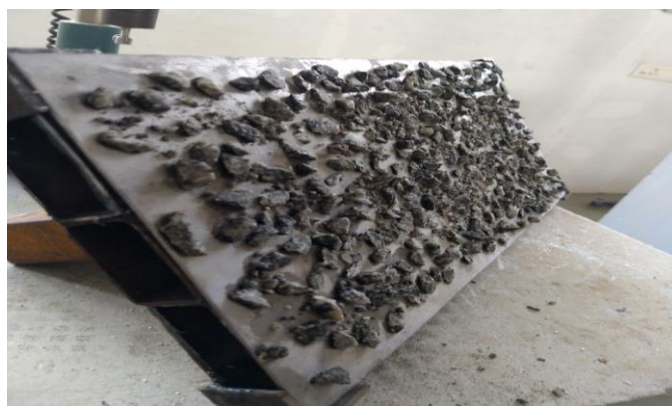
Fig 2-Rough surface under footing
