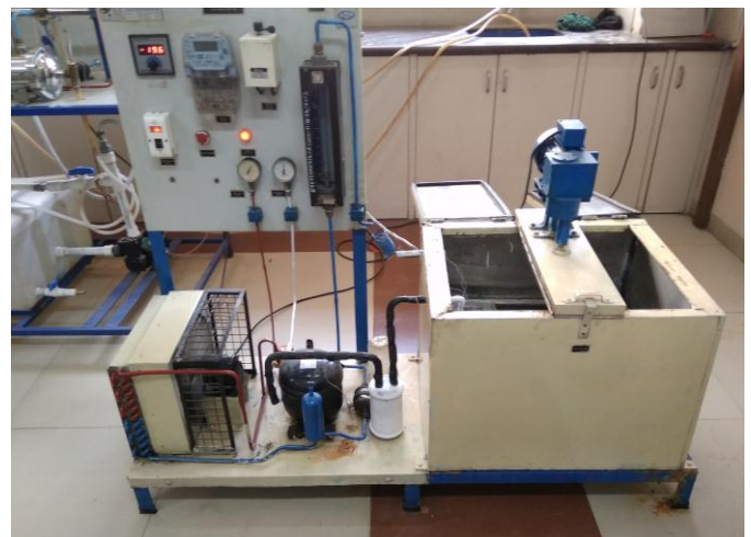
Fig -3: Ice plant test rig
