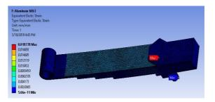
The maximum equivalent strain for the Al 6063 can be observed as 0.018778. The condition of the designed leaf spring is meant to be safe as most of the part of the leaf spring observes minimum strain which is equivalent to zero MPa. The above image concludes that only limited part of the leaf spring is subjected to maximum strain of 0.018778 while majority of the leaf spring stays under the fatigue level.
