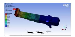
The maximum equivalent strain for the Al 6061 can be observed as 0.018012. The condition of the designed leaf spring is meant to be safe as most of the part of the leaf spring observes minimum strain which is equivalent to zero MPa. The above image concludes that only limited part of the leaf spring is subjected to maximum strain of 0.018012 while majority of the leaf spring stays under the fatigue level.
