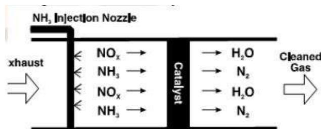
Figure 4: Selective Catalytic Reduction
