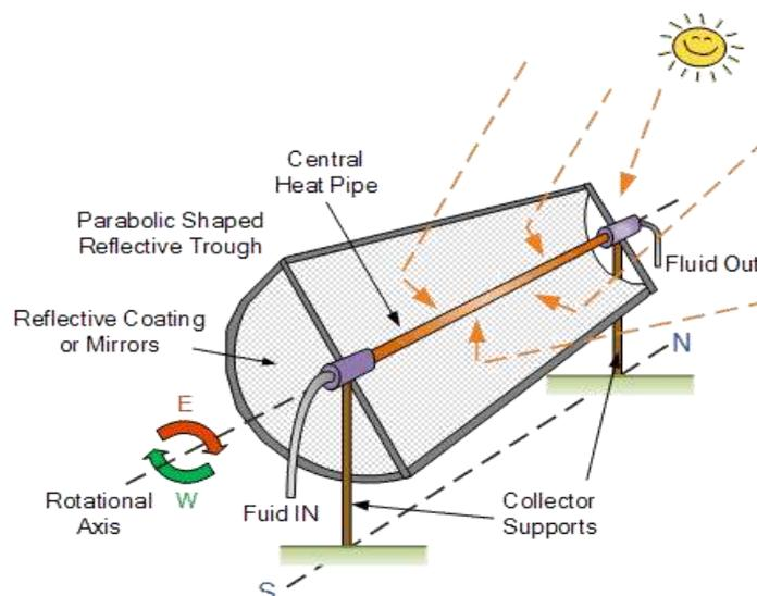
. Fig. Schematic diagram of Parabolic Trough Concentrator
