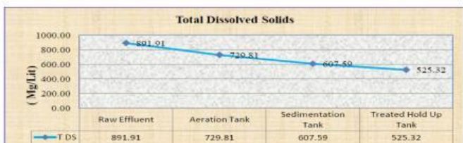
Variation of Total Dissolved Solids at different units (components) of ETP.
