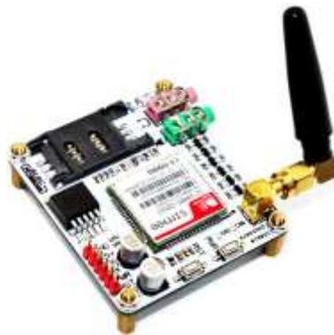
GSM Module is a device which used to send a message from one device to another device.
