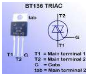
Fig 2.4: Pin Diagram of BT136 Triac
